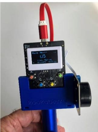
This [MoveMusic App](#) uses the Kookaberry's accelerometer (all smartphones and tablets have one – it is what makes the screen rotate to suit your viewing angle) to play the scale of C Major in the seven octaves of a standard piano.
